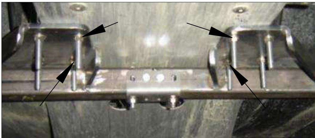
Attach well the plate 03PA-264 to the frame .
