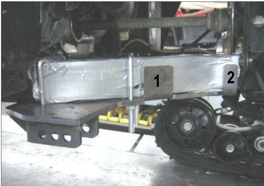
Once the guard is trimmed, put both bends along the frame (1-2 above).
